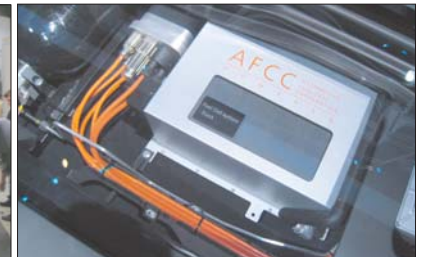
Main components: Fuel Cell Stack detail
