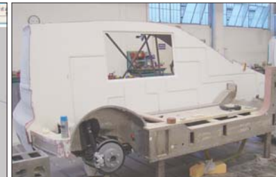
Body construction ( glassfiber )
