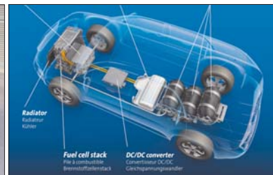
Virtual animation: main Hydrogen 4 Hybrid components description
