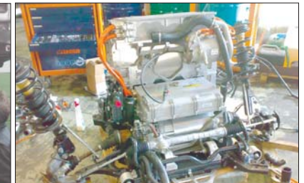
Hydrogen 4 powertrain FC details
